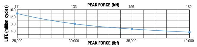
**NOTE:** The L10 life estimation method does not include failures caused by other conditions such as contamination, misalignment, improper lubrication and exceeding actuator specifications
