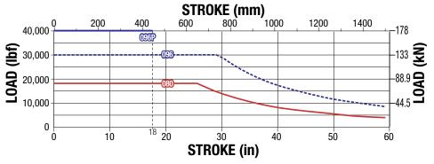
\*NOTE: When using Trunnion Mount, (TRR) consider the stroke to be longer when determining Critical Speed and Buckling Load:
