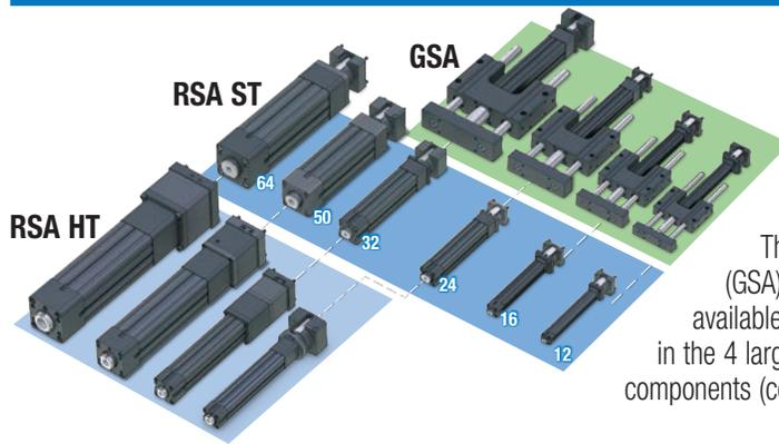
The RSA is a flexible electric screw driven rod-style actuator. The standard (ST) model comes in six sizes. The guided RSA (GSA) adds guidance and load support to the design and is available in the 4 smaller sizes. The high force (HT) model is available in the 4 larger sizes, it incorporates stronger torque transmission components (couplers, pulleys, belts) and higher thrust bearings.
